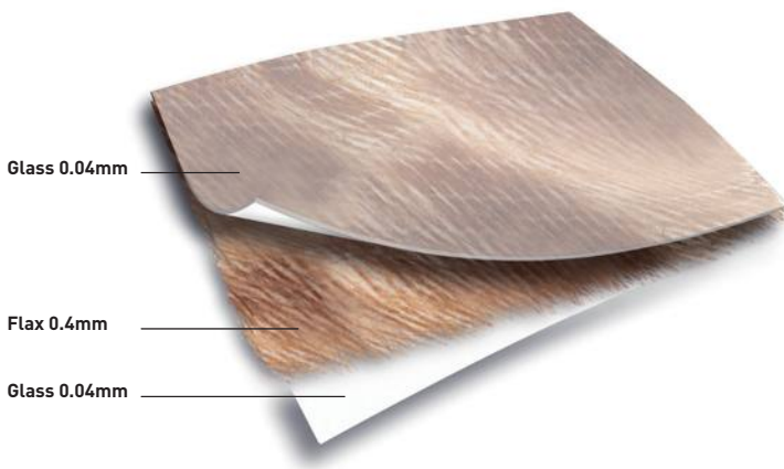
Flax sandwich Details for midrange driver
